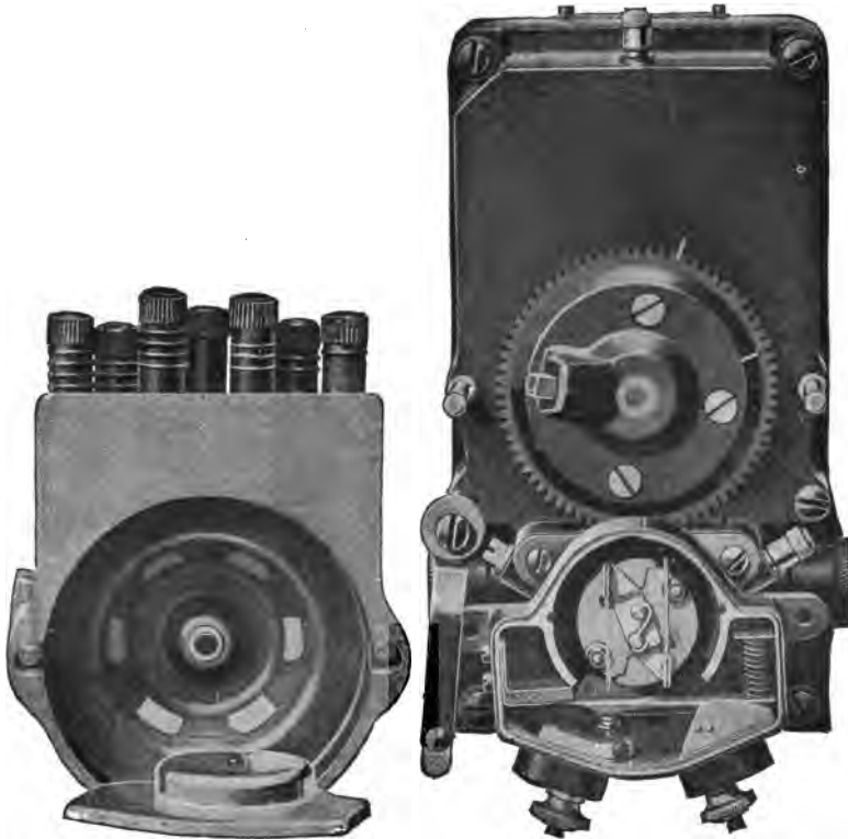
FIG. 54.—Westinghouse distributor and interrupter cover removed. Position of centrifugal weights with engine idle.
